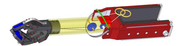
Fig. 10.15. Detailed assembly diagram of the final transhumeral device.
